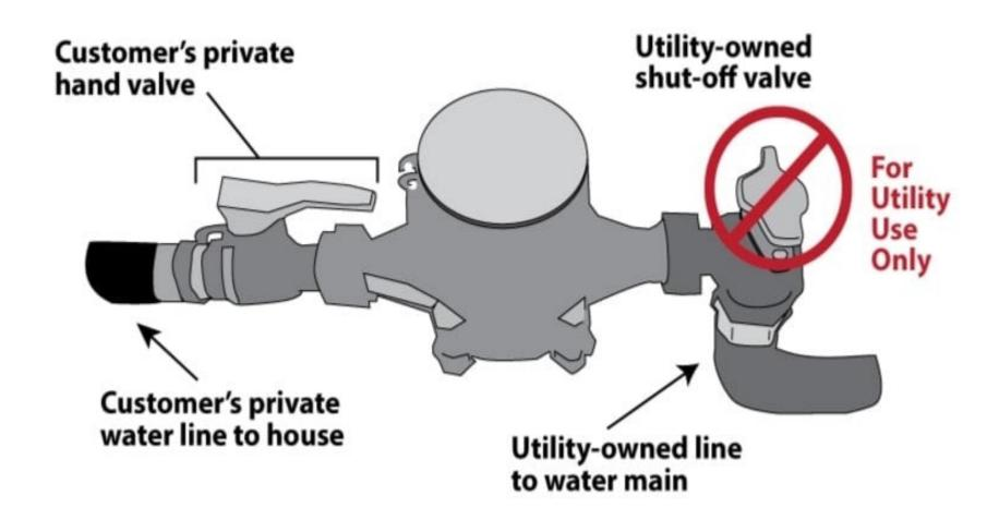
Diagram to show where customer shut off valve should be located.
